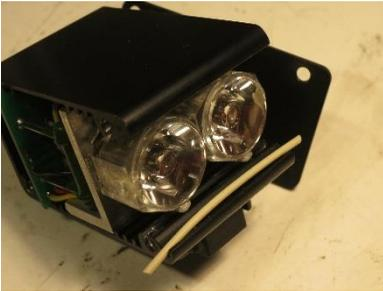
Lay the rubber seal in to the bottom front window groove. Leave a few millimetres sticking out of one end, and cut off the other end also leaving a few millimetres sticking out.
