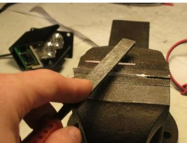
Clamp the window firmly in a vice, using some paper or similar to stop it getting scratched, and file away the marked area. Make sure the edge you leave is straight and smooth, because it has to form a good seal. Use fine emery paper or wet-and-dry paper if necessary.
