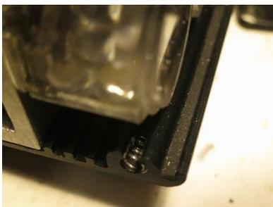
If the seals are the black neoprene foam type, they may have been crushed so much that they are almost invisible. The seals are self-adhesive and may be firmly stuck to the inside of the grooves in the light.
