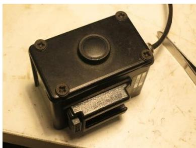
Do not overtighten the screws: tighten them only until the side panel is held snugly in position. Overtightening will push the o-rings out of place.
