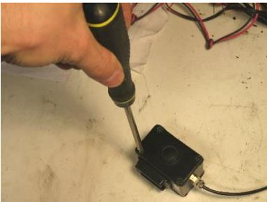
Remove both side panels from the light by unscrewing all eight of the screws.
