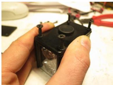
Carefully insert each screw. You may have to squeeze the case together, either by hand or in a vice, to get the screw holes to line up with those in the side panel. As you turn the screws, make sure the gasket doesn't get twisted out of place. Squeezing the side panel against the case will help to hold the gasket in position.
