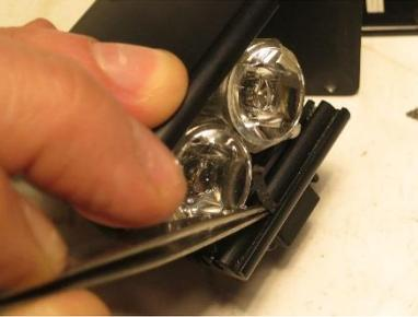
Carefully scrape away all traces of the old seals using a tiny screwdriver or tweezers. Gentle heat may help.
