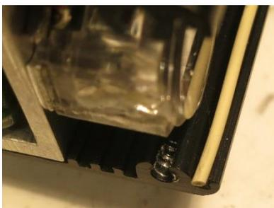
If they are the pale yellow-coloured silicone rubber type, no modifications are necessary. Simply remove and discard the old seals ready to fit new ones later.
