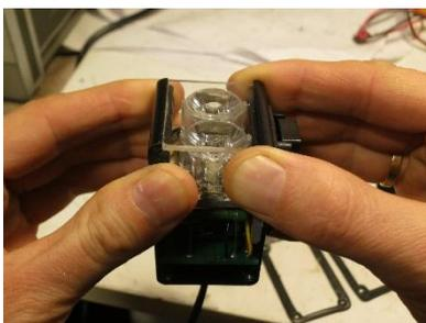
Gently pull apart the front of the light by hand and slide out the front window.
