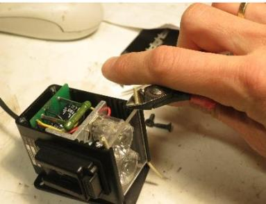
Use sharp flush cutters or a craft knife to cut off the ends of the seals, leaving about half a millimetre sticking out.
