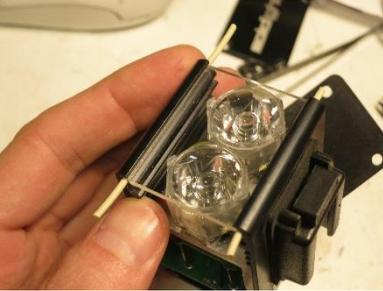
Gently pull the casing apart to allow the window to get into the groove on top of the seal. The springiness of the case will hold everything in place.
