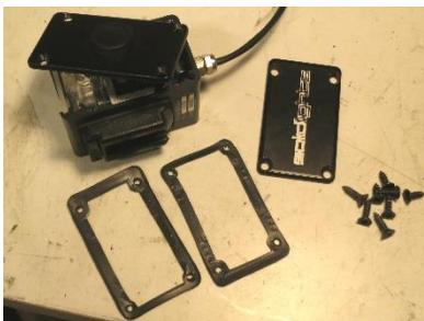
Discard the old screws and o-rings, if fitted, but keep the two rectangular gaskets. One side panel will remain attached to the light by the wiring to the button. Take great care not to damage the wiring by pulling or bending it excessively.
