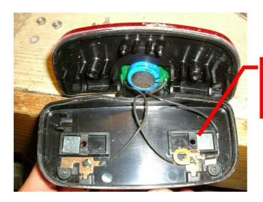
The part has now been cut off so the mounting screw fits into its hole and doesn't contact the copper part and, thus, the wiring.
