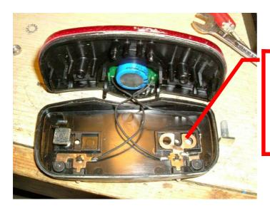
This copper-coloured part makes the connection between the mounting screw (removed here, lying to the right of the light) and one of the wires.
